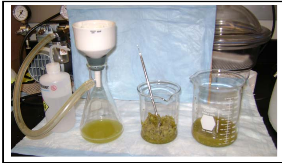
Figure 6.2 Cactus pad preparation showing vacuum filtration apparatus
